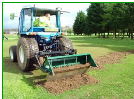
DUMPS AUTOMATICALY WHEN RAISED
